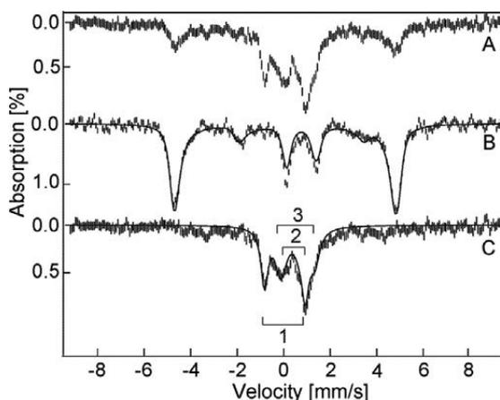
FIGURE 2. Mössbauer spectra of  $^{57}\text{Fe}$ -TDO. A, reaction of  $\text{H}_2\text{O}_2$  (9.6 mM) with TDO (1.6 mM); B, TDO protein in resting state prior to the reaction with  $\text{H}_2\text{O}_2$ ; and C, difference spectrum of  $A - 0.25B$ . All spectra were recorded at 4.2 K in an applied field of 45 mT parallel to the direction of the beam of  $\gamma$  rays. The solid lines are least squares fits with parameters given in the text.
