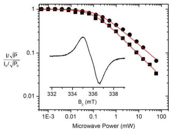
**Figure S5.** The  $g = 2.0028$  free radical (inset) and its relaxation properties. The power saturation of the 10 K (■) and 100 K (●) and the fit to Eq. 2 are shown, where  $I$  is the EPR signal amplitude and  $P$  is the microwave power.
