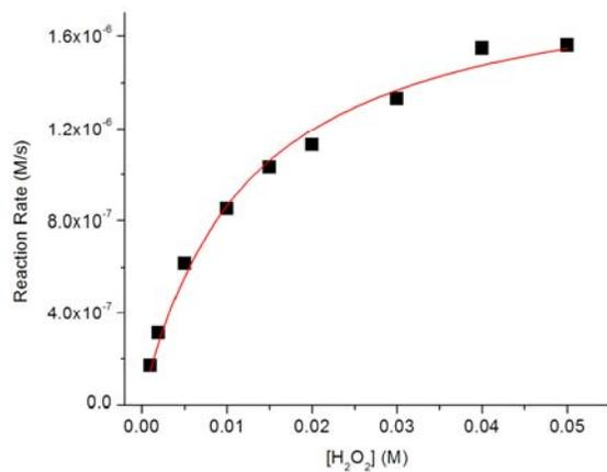
**Figure S2.** Top Panel: Saturation curve showing the relation between the concentration of H<sub>2</sub>O<sub>2</sub> and rate of the catalase-like activity of ferric TDO. Three repeating experiments were carried out and similar results were observed.
