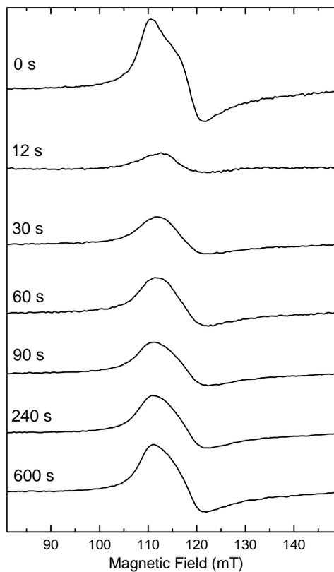
**Figure S3.** EPR spectra of the high-spin ferric heme ( $150 \mu\text{M}$ ) taken during the reaction with  $\text{H}_2\text{O}_2$  ( $900 \mu\text{M}$ ). EPR parameters: recording temperature, 10 K; microwave power, 1 mW; microwave frequency, 9.44 GHz; modulation amplitude, 0.8 mT.
