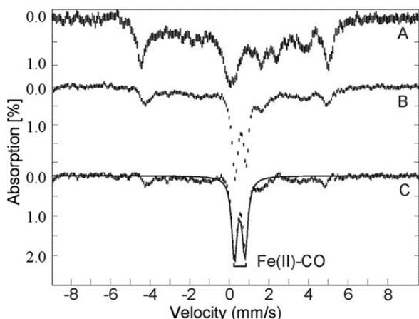
FIGURE 6. Mössbauer spectra of  $^{57}\text{Fe}$ -TDO. A, ferric TDO (1 mM) with 50 eq of L-Trp; B, after treatment with CO and  $\text{H}_2\text{O}_2$  (2 mM); and C, difference spectrum of B - 0.5A. All spectra were recorded at 4.2 K in an applied field of 45 mT parallel to the direction of the beam of  $\gamma$  rays. The solid line is the least squares fit with parameters given in the text.
