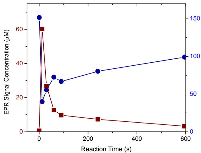
**Figure S4.** EPR signal intensity as a function of reaction time for the  $g = 2.0028$  (wine trace, ■) and  $g = 6$  (navy, ●) resonances, respectively. The initial heme concentration was  $150 \mu\text{M}$ .
