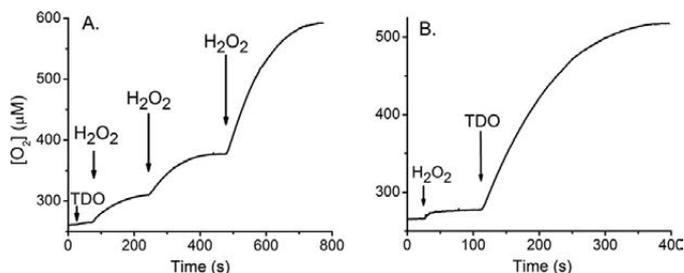
FIGURE 1. A,  $\text{H}_2\text{O}_2$  decomposition and  $\text{O}_2$  production mediated by  $\text{Fe}(\text{III})$ -TDO in a stirred  $\text{O}_2$  electrode cell in response to discrete additions of  $\text{H}_2\text{O}_2$ . B, reaction initiated by TDO. Arrows indicate the time points in which ferric TDO (5  $\mu\text{M}$ ) and  $\text{H}_2\text{O}_2$  (250  $\mu\text{M}$  or 1 mM in A and 1 mM in B) were added to the reaction cell.
