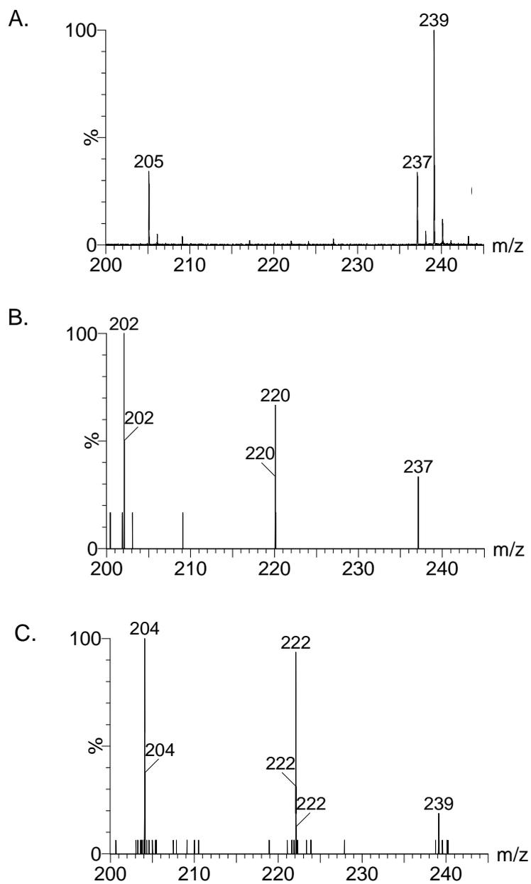
**Figure S9.** MS/MS analysis of  $m/z$  220 and  $m/z$  222 ion peaks. (A) ESI-MS spectrum of the TDO reaction in  $\text{H}_2^{18}\text{O}$  solvent. MS/MS characterization of ion peaks of  $m/z$  237 (B) and  $m/z$  239 (C) of the spectrum A, respectively.
