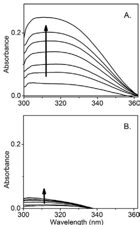
FIGURE 5. Formation of NFK as a result of the peroxide reaction with ferric TDO (5  $\mu\text{M}$ ) and L-Trp (5 mM). The spectra were taken from the anaerobic titration of 35 eq of  $\text{H}_2\text{O}_2$  (total 175  $\mu\text{M}$ ) in the absence (A) and presence (B) of hydroxyurea (10 mM). Each trace was obtained after the reaction was complete and subtracted against a spectrum of ferric TDO at the same concentration (5  $\mu\text{M}$ ).
