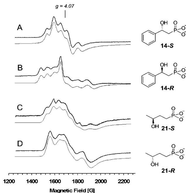
FIGURE 7: EPR spectra of Fe(II)-HppE-nitrosyl complexes with different substrate analogues. (A) (*S*)-HPEP (**14-S**); (B) (*R*)-HPEP (**14-R**); (C) (*S*)-HBP (**21-S**); (D) (*R*)-HBP (**21-R**). Instrumental parameters are the same as shown in Figure 3. Gray lines represent simulated spectra.
