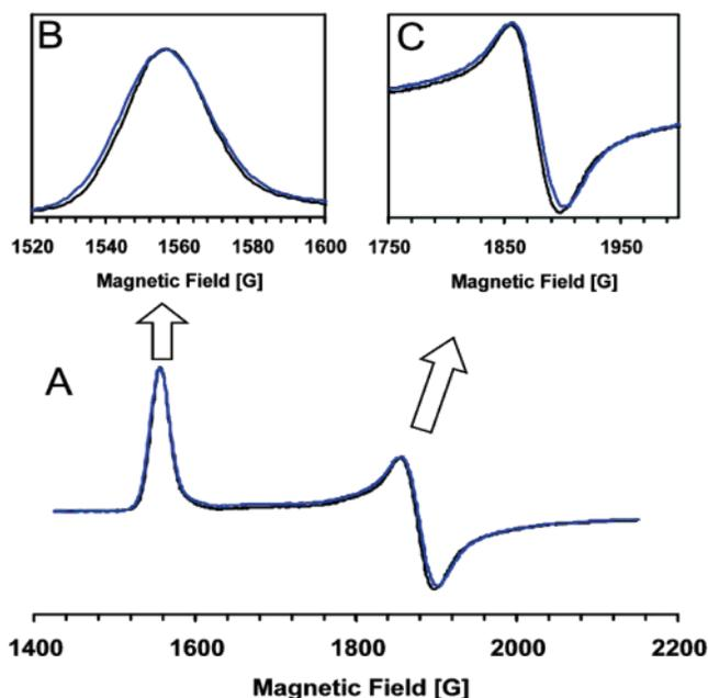
FIGURE 5: EPR spectra of Fe(II)–HppE nitrosyl complex with (*R*)-[<sup>17</sup>O]HPP (**12-R**). Panel A: full low field region of the spectrum; Panel B: detailed view of the  $g = 4.42$  region; Panel C: detailed view of the  $g = 3.63$  region. Black lines: (*R*)-[<sup>16</sup>O]HPP; Blue lines: (*R*)-[<sup>17</sup>O]HPP. Instrumental parameters are the same as shown in Figure 3.
