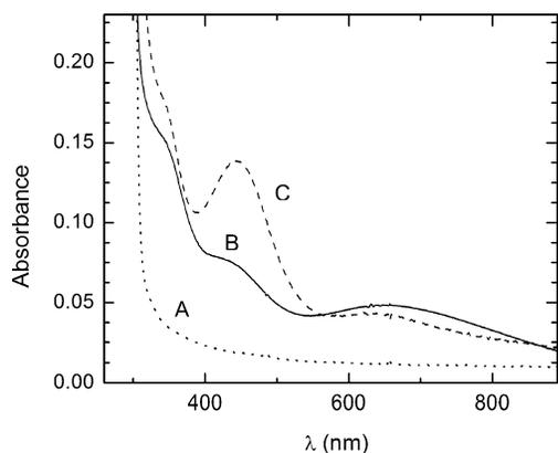
FIGURE 2: Electronic absorption spectra of Fe(II)–HppE nitrosyl complexes. (A) As-isolated HppE (200  $\mu$ M) (metal-free); (B) HppE (180  $\mu$ M) reconstituted with Fe(II) and exposed to NO; (C) to sample B was added (S)-HPP (4 mM).
